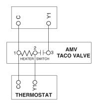
Fig. 32 — AMV Valve Wiring
